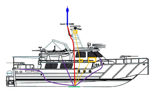
**Figure 1:** Simple installation example for vessels. Key: Blue = Stormaster ESE air terminal and FRP insulated support mast; Red = HVSC Plus lightning downconductor cable; Green = earthing plate / zinc anode; Purple = bonding conductors (representative only); Orange = surge protection.
