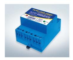
Series powerline protection is the best available protection for sensitive electronics such as rectifiers, switchmode power supplies, and other mission critical equipment. The Series Filter reduces the rate of rise of any transient overvoltage to acceptable levels, and also reduces the overall magnitude of the transient voltage the equipment receives.
