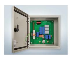
Standard Surge Filter Order Code: SF X YY ZZZ-100+50-AIMCB Where X is the number of phases, YY is circuit current rating per phase, ZZZ is the voltage. Standard filters are manufactured and supplied 100 kA line and 50 kA load size. All surge filters are supplied with Alarm interface module (AIM).
