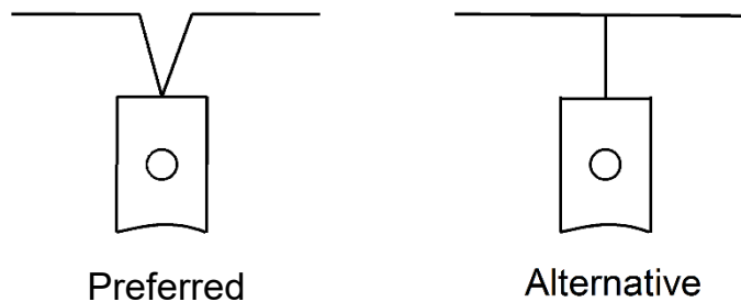
Figure 2: Connection methods. (a) V (Kelvin) connection (preferred). (b) T connection (alternative).
