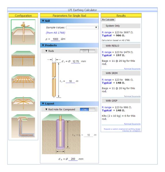
Working left to right, select the configuration of the earthing system, then edit the dimensions and other parameters. Results are given for the theoretical best-case scenario (as per the standard) as well as likely real-world values as typically seen in the field
